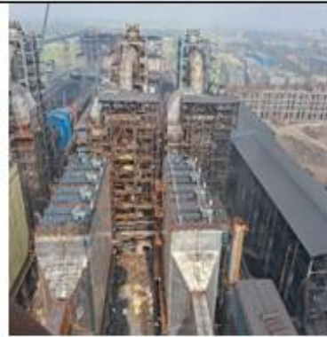
ESP for arresting dust emission in DRI Plant (2 x 350 TPD + 2 x 500 TPD)
